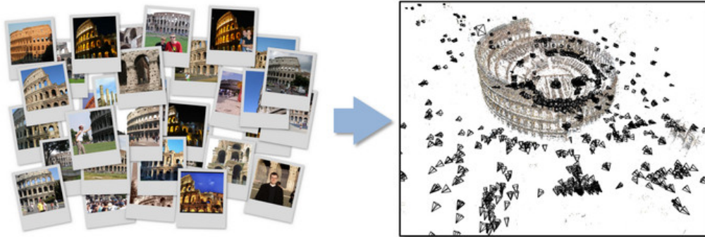
Figure 3: The structure from motion system registers unordered images and produces a sparse point cloud.
